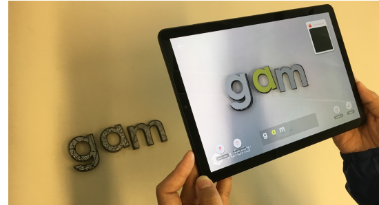
Figure 4. A demo of the Visual Markers-based technique overlaying physical letters with their digital representations.
