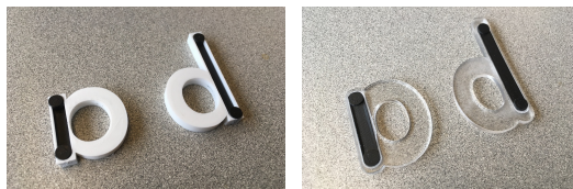
Figure 7. Iterations of capacitive letters (back side of 'a' and 'b'). 3D printed letters and pads (Left), laser-cut & engraved letters and 3D printed pads (Right).
